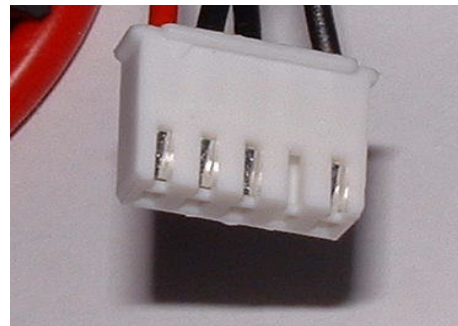
The very useful external connector for checking and balancing your pack
