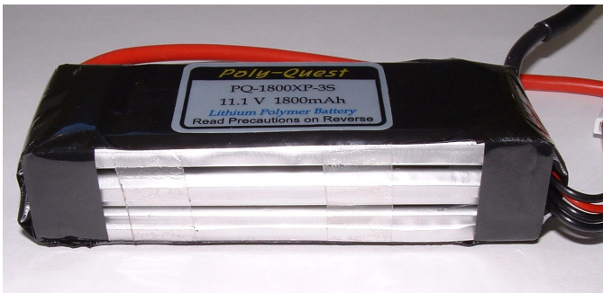
Side view of the pack showing the space between the cells
